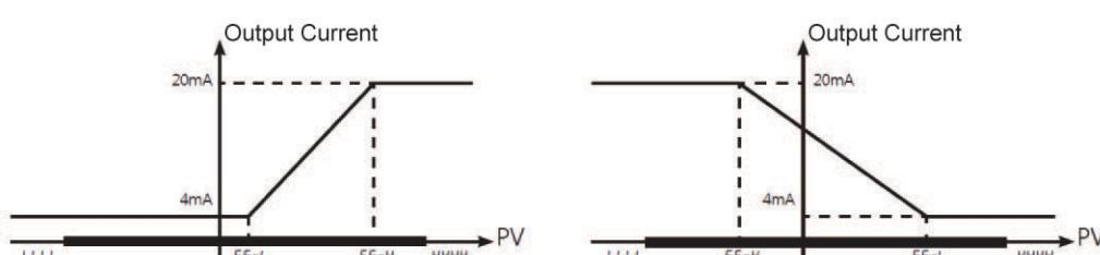
\* : Sensor Range or High/Low-limit Scale
